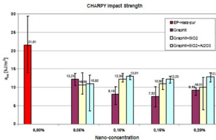
**Fig.9 Comparison of CHARPY Impact Strength**
