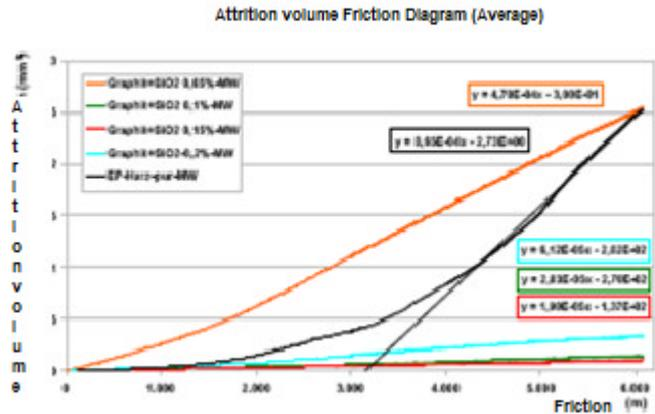
Fig.5 Attrition Volume of ER- resin with different concentrations of the mixture of graphite and SiO<sub>2</sub>
