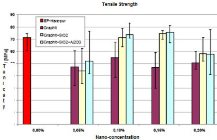
Fig. 10: Comparison of tensile strength
