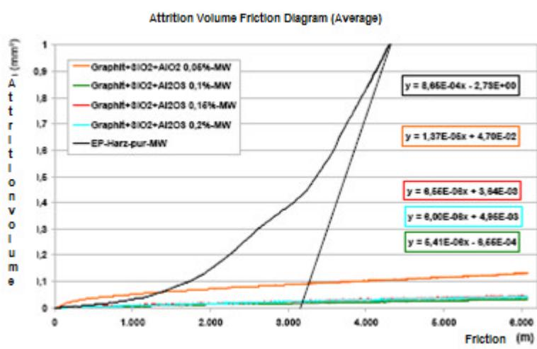
Fig.6: Attrition volume of ER-resin with different concentrations of graphite/SiO<sub>2</sub>/Al<sub>2</sub>O<sub>3</sub>
