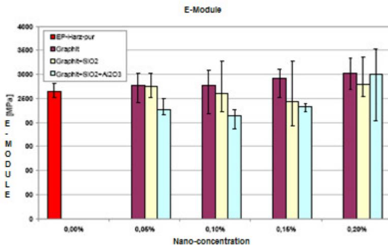
Fig.12: Comparison of E-Modules
