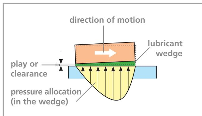
Picture 1: The formation of a lubricant wedge
