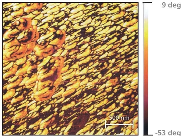
Picture 3: Electrical polarized nano-powder
