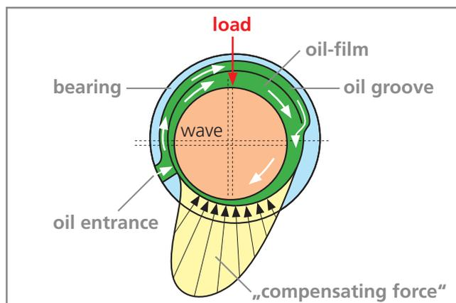
Picture 2: The load-spread in a plain bearing
